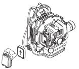
An air filter that has been in use for a long time cannot be cleaned completely. The filter must therefore be replaced with a new one at regular intervals. A damaged air filter must always be replaced.
