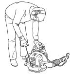
Repeat pulling the cord until the engine starts. When the engine starts, return choke control to run position.
